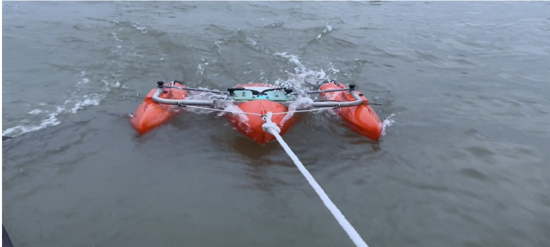
Figure 9.1: Discharge Measurement in Ganga River using ADCP Measurements using Acoustic Doppler Current Profilers (ADCP)
