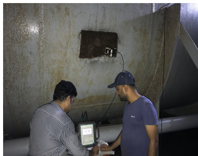
Figure 5.24: On-Site Efficiency evaluation for Francis turbines of Koyna Stage IV
