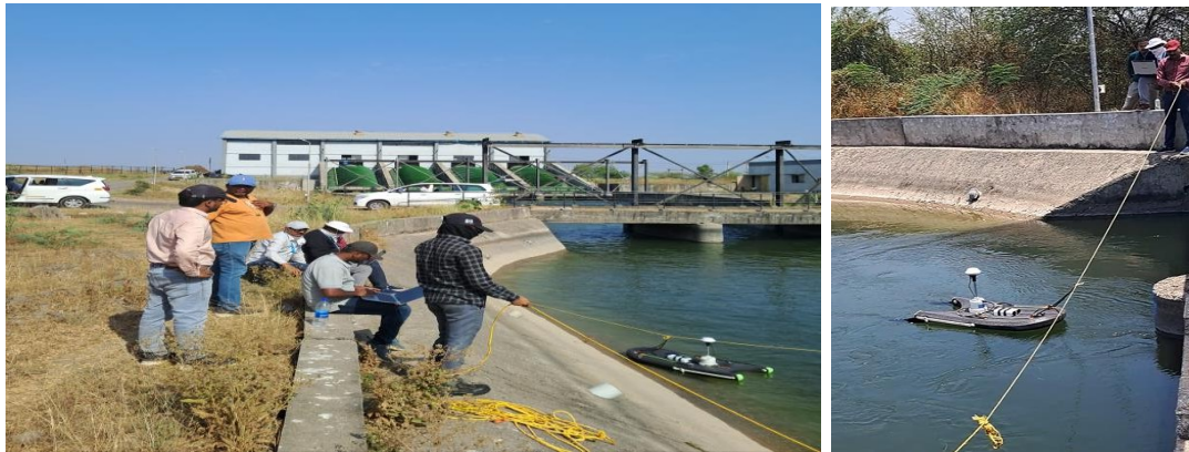
Figure 9.3: Onsite Efficiency Test of Screw Turbine Plants in Canal of SSNNL
