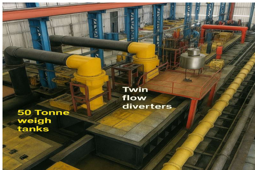
Figure 3.1: Gravimetric Calibration Laboratory at CWPRS
